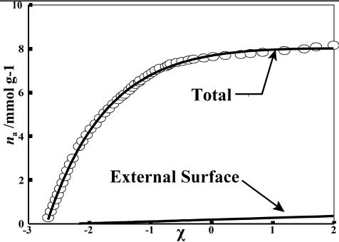
**Figure 33** The fit to the ND data including the log-law, mainly, followed by the linear fit for external adsorption. The  $\chi$ -plot is used to show both high and low pressure reagions. Compare this to **Figure 3**
